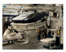
**IMPROVED HOPPER AREA:** Big step for easier cleanout. New bracket for water hose.
