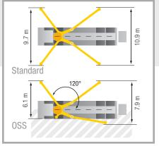
Country-specific admission requirements for 4 or 5 axles must be checked. Dimensions are model-dependent and may vary. Gross weight depending on equipment and chassis  $\leq 40 \text{ t}$
